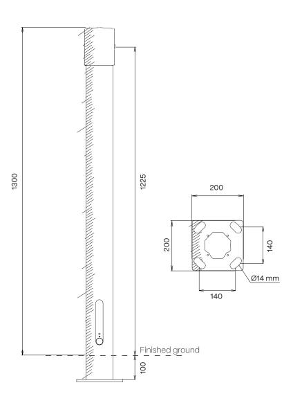
• Easy installation and removal using a screw-in base, 140x140 mm spacing
