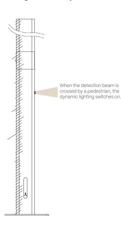
At night, the dynamic lighting shows warning markings on the S-Pass+ column and the lights on the tops of the S-Pass bollards flash.
